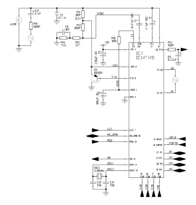
Figure 2: Equivalent Test Circuit
