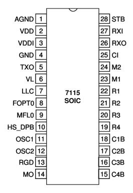
Figure 1: 28-lead SOIC Package
